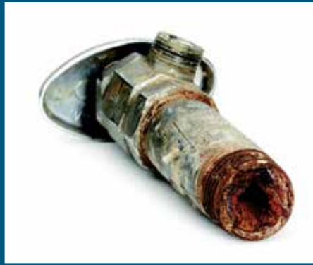
B. Galvanized pipe corrosion
